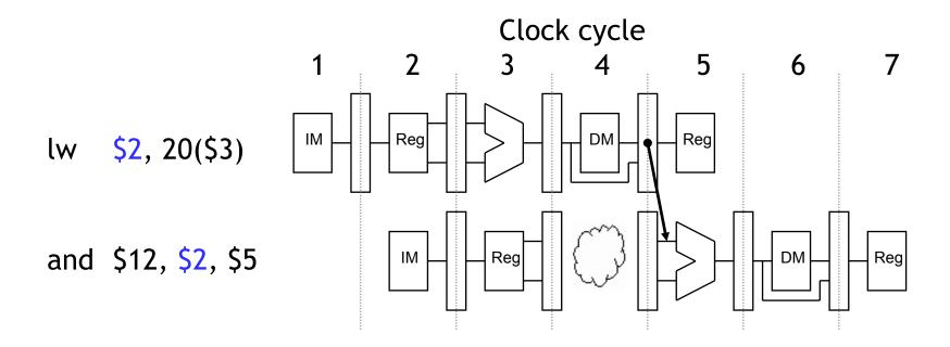
Notice that we're still using forwarding in cycle 5, to get data from the MEM/WB pipeline register to the ALU.
